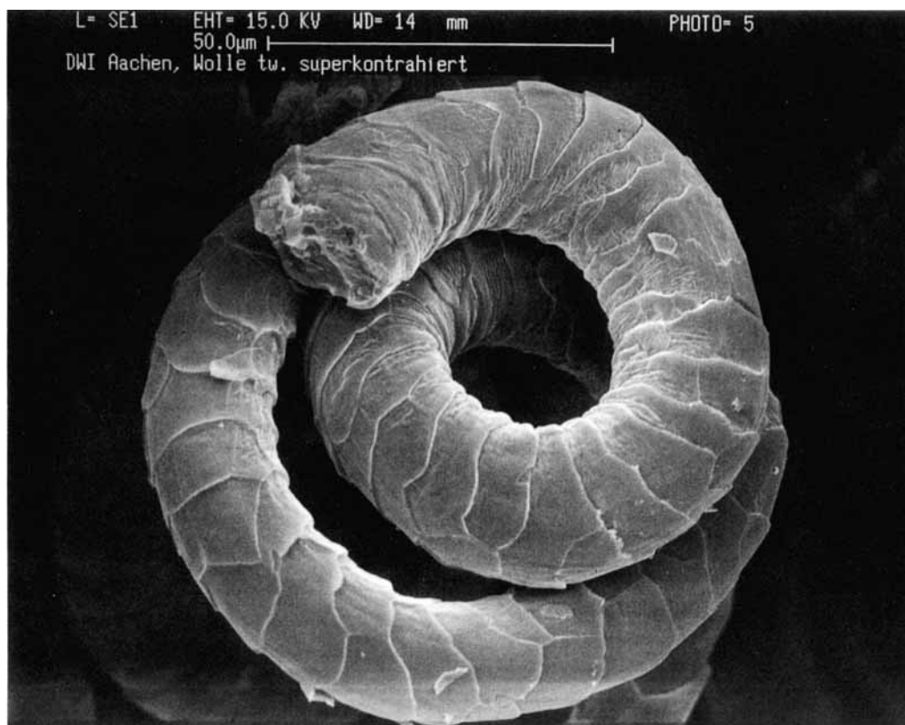
Figure 11 SEM micrograph of a merino wool fiber, differentially supercontracted by HPDSC.
